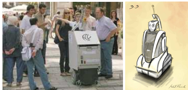
Figure 1: ACE, the precursor to IURO (left) and a design draft of the IURO robot (right).
